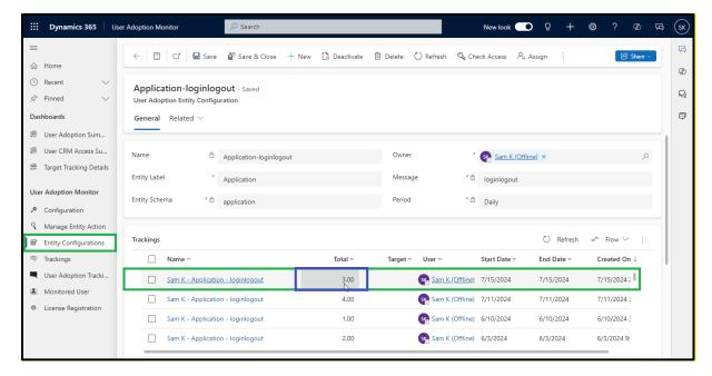
Here, under the "**Total**" tab, you can see that the value increases with each action performed by Sam. Each time a user logs in or out of the application, the action count will go up.
